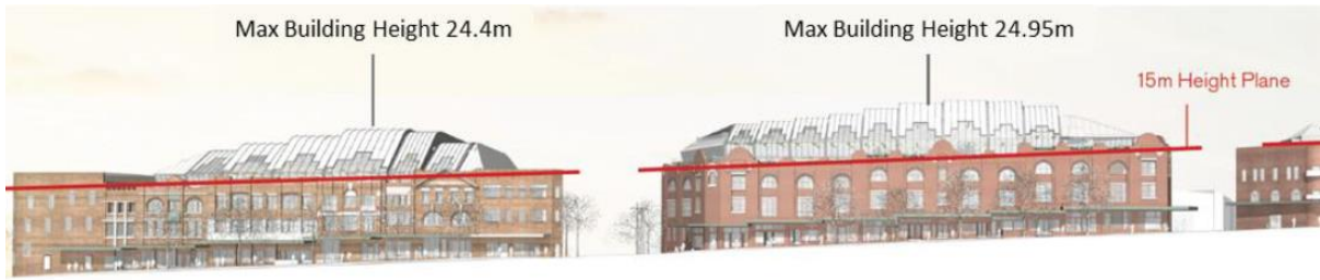
Figure 17: Elevation drawings of Groups 1 and 2, with the 15 metre Sydney LEP 2012 height control shown in red, as viewed from Oxford Street (Note: this image has not been amended since the roof forms have changed, however the heights have not increased)
